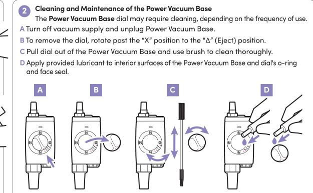
Return dial to installed position in Power Vacuum Base.
