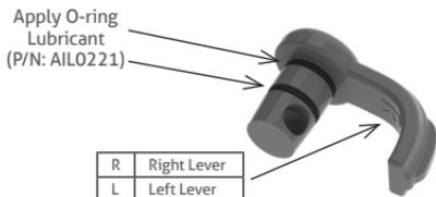
Figure 10. Vacuum Lever to Lubricate
